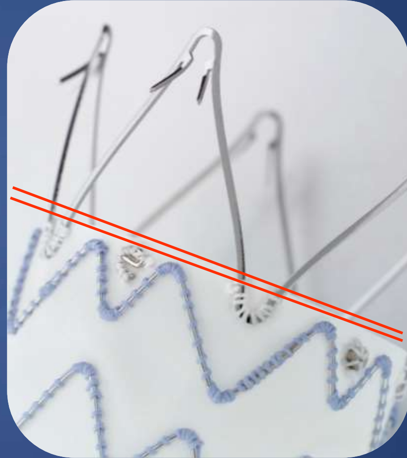
Proximal edge of stent graft 1mm above proximal markers
